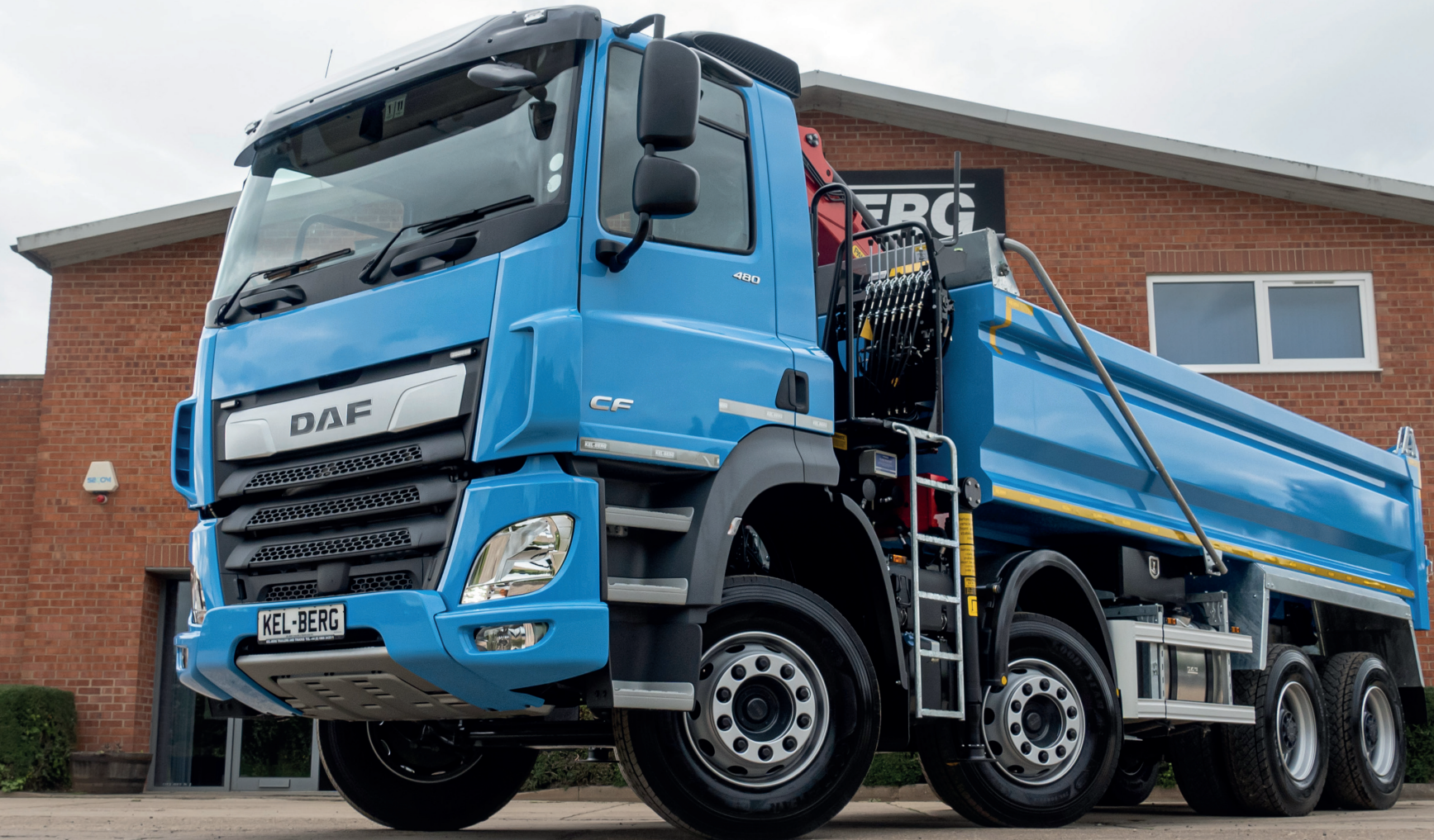
DAF CF480 8x4 Day Cab c/w Kel-Berg Grab Loader Installation + Drawbar
